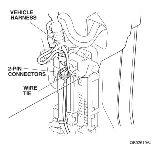
43. Bundle up the excess door sill trim harness, and secure it to the vehicle harness with one wire tie.
