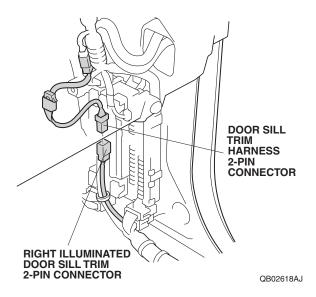
42. Secure the 2-pin connectors to the vehicle harness with one wire tie.
