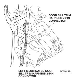
34. Bundle up the excess door sill trim harness, and secure it and 2-pin connectors to the vehicle harness with one wire tie.
