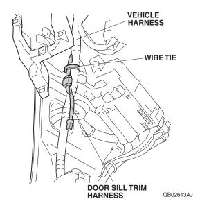
33. Plug the door sill trim harness 2-pin connector into the left illuminated door sill trim harness 2-pin connector.
