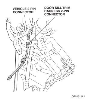
32. Secure the door sill trim harness to the vehicle harness with one wire tie.
