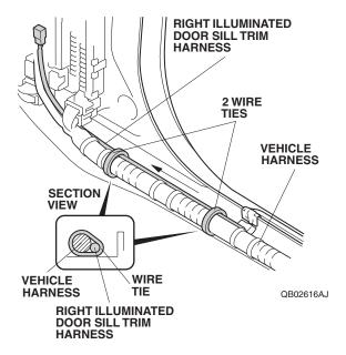
36. Secure the right illuminated door sill trim harness to the vehicle harness with two wire ties.
