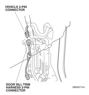
41. Plug the door sill trim harness 2-pin connector into the right illuminated door sill trim harness 2-pin connector.
